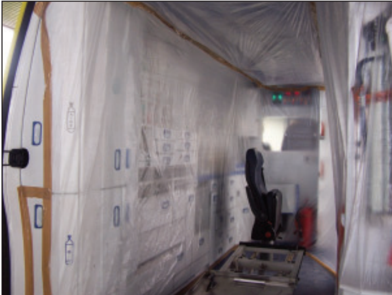
Figure 3. The inside surfaces of the vehicle are covered in order to reduce the risk of contamination.
